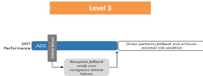
Figure 2 - Use case sequence at Level 3 showing ADS engaged, a vehicle failure and the user resuming control
