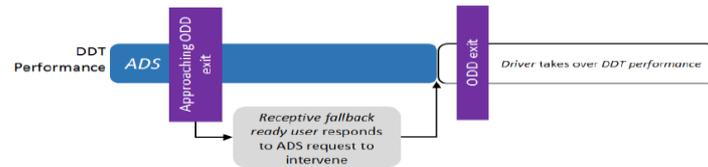
Figure 4 - Use case sequence at Level 3 showing ADS engaged, exiting the ODD and the user resuming control
