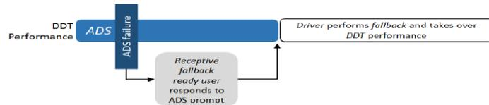
Figure 3 - Use case sequence at Level 3 showing ADS engaged, and ADS failure and the user resuming control
